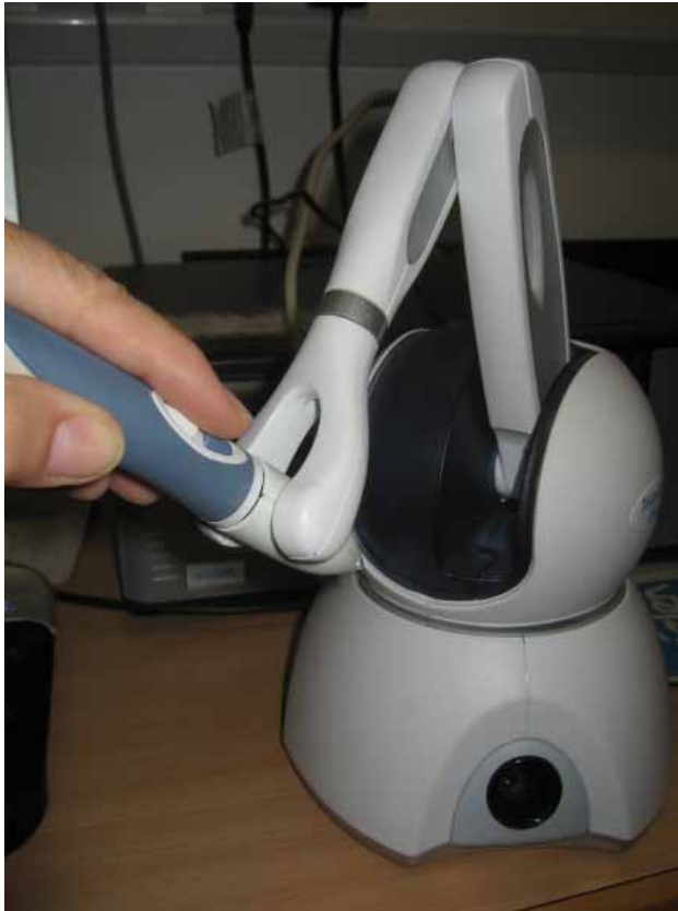
Figure 7. Haptic tool: the Phantom Sense-Abel
